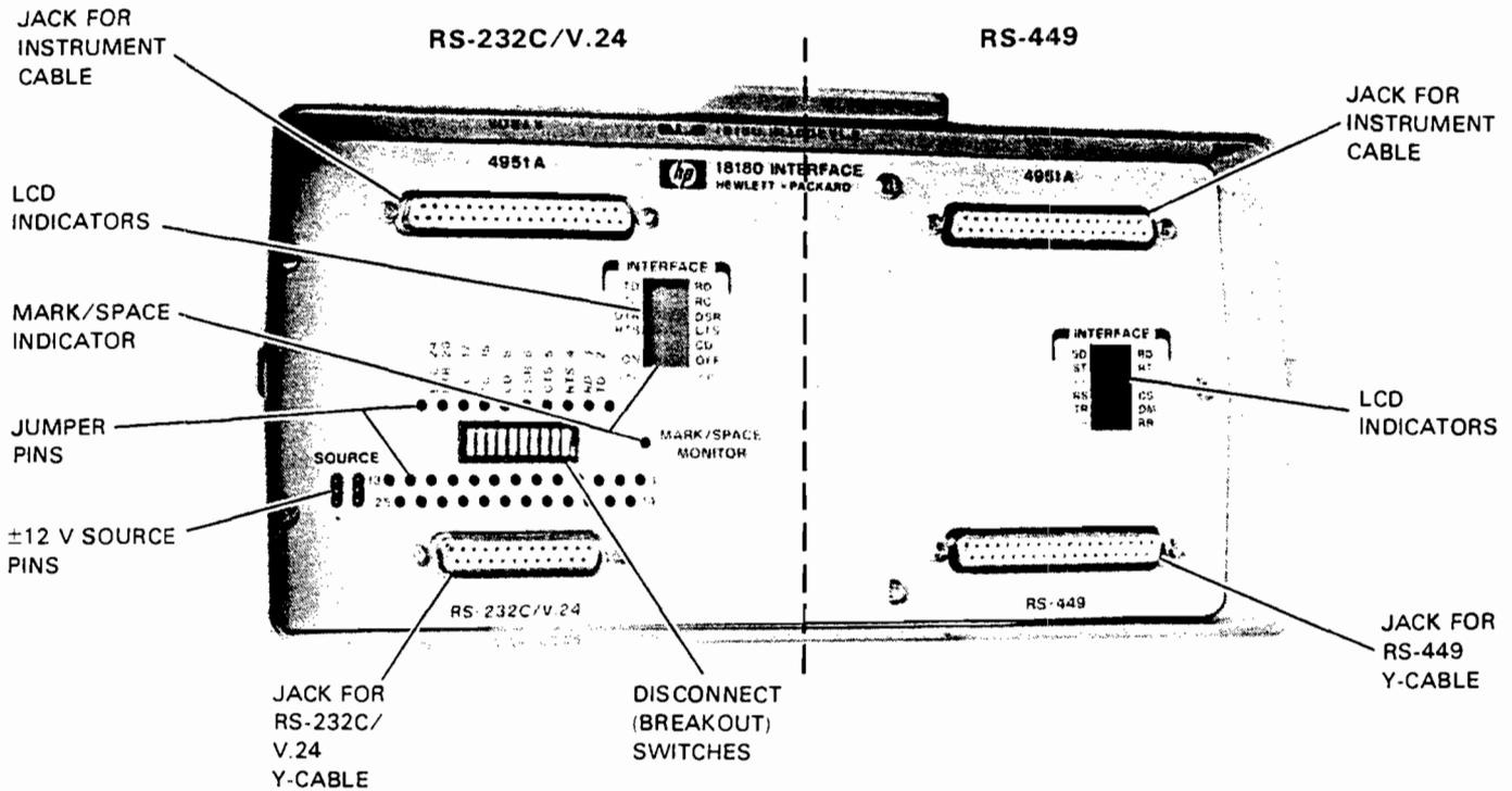
Figure C-1. The HP 18180A (Combination RS-232C/V.24 and RS-449 Interface)
