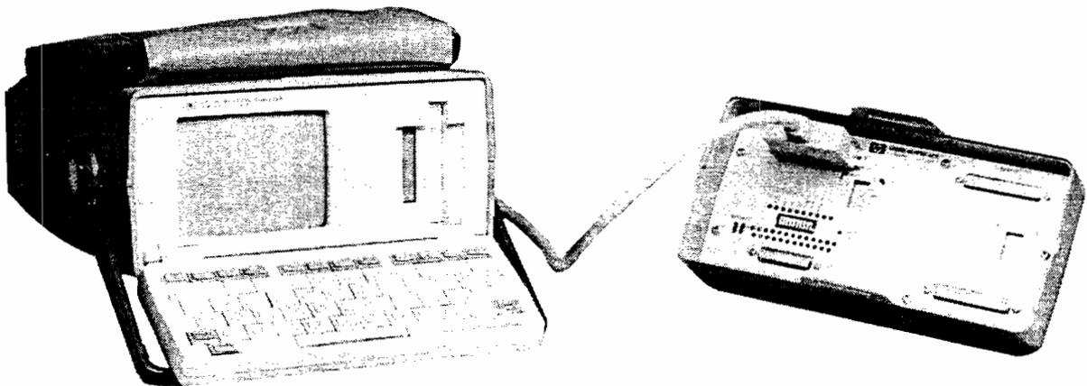
Figure 3-1. Hooking Up the Interface Pod
