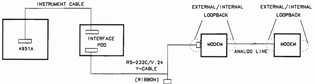
**Figure 9-3. Loopback Testing**
