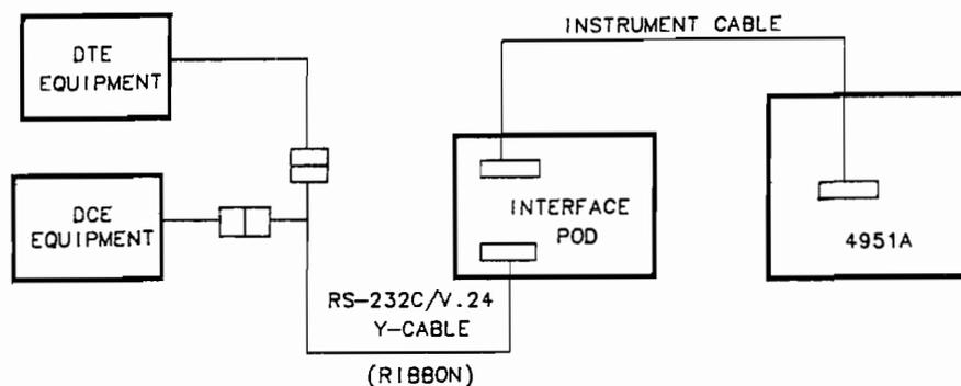
Figure 2-1. Hookup for Line Monitoring
