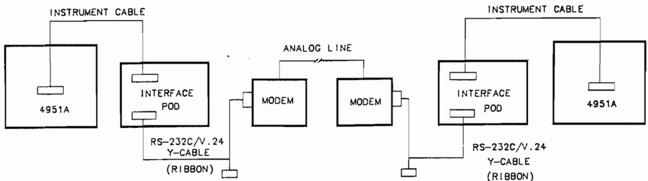
Figure 9-2. End-to-End Testing
