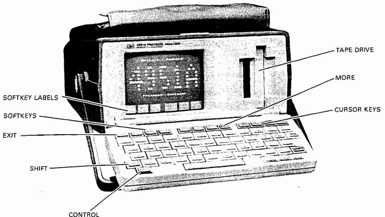
Figure 1-2. Front Panel Controls
