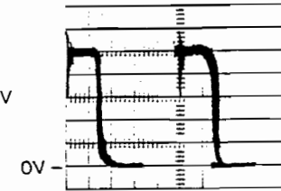
CR6 anode 2 μsec/Div 5 V/Div, DC coupled
