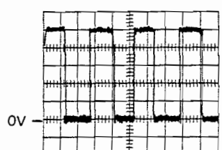
A3U404 pin 10 10 \mu sec/Div 1 V/Div, DC coupled
