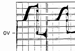
CR8 (anode) 2 μsec/Div V/cm 20, DC coupled
