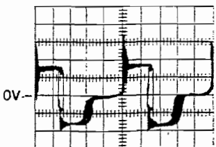
CR9 (anode) 2 μsec/Div 10 V/Div, DC coupled
